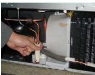
Make a space to pull out bell mouth by pushing dryer lightly which is located in front of a bell mouth to a compressor side.
