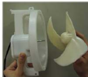
Separate a blade of a fan from a C-Fan motor shaft.
