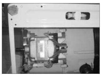
4) Remove the motor from the tub.
