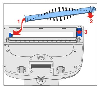
To replace the Brush Motor (15), Driving belt (12) and Roller Holder assy (13):
