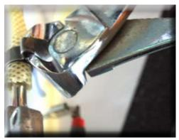
Use a suitable pair of pliers to remove the clamp (as shown).
