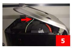
**5)** Lift the upper cover and disconnect the earth wire shown.
