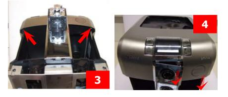
**3**) Loosen the screws shown from inside the compartments that contain the water tank and dreg drawer.
