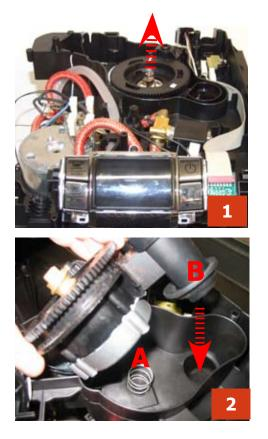
**1)** To remove the coffee grinder, simply slide it out and remove the connections.
