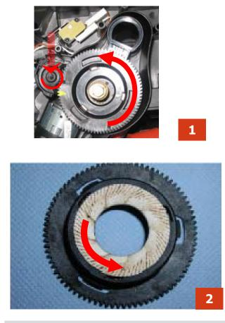
**1)** To remove the upper grinder blade support, use an Allen wrench and turn it clockwise to release it from the bayonet coupling.
