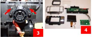
**1**) Loosen the screw shown and remove the cover, glass panel, frame, keyboard and seal.
