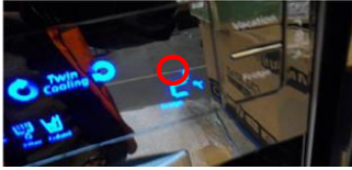
[ LED segment manquant sur RSH*]
